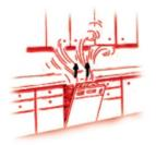
Wait approx. 20 minutes before opening the dishwasher at the end of its program so that the steam can condense out inside the machine.
